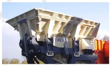
The folding walls cylinders are housed under a special guards.
