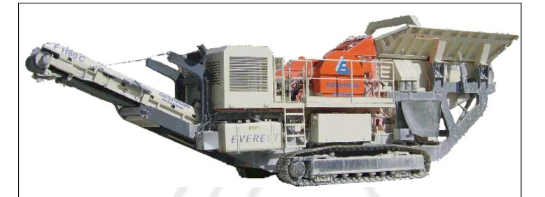
The model **CRUSHER TRACK EVEREST** is one of the biggest mobile crusher in the Gasparin Omg product range, equipped with last generation management systems, it is easy to use and environmentally freindly. Made for any quarry application (including very hard rock), good as well in recycling application.
